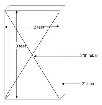
Note: 3/8" (inches) rebar to be used as illustrated; to reinforce the concrete non-slip surface is required.
